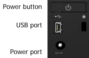
Figure 1. USB ports on a USB hard drive
